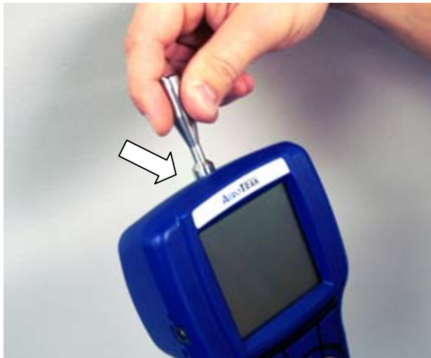
Installing an Isokinetic Inlet
